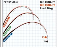
Static load comparison of BIG TUNA 76 and BIG TUNA 73 (10kg load) These models will assist anglers for situations where large lures are required due to the targets feeding on large baits such as dolphin fish. At a  $45^\circ angle,$  both the 73 and 76 can be seen to have the same power. However, once the rod is lifted even higher, the 76 will start bending closer to the body, reducing the load on the angler. The 73 has a sharp casting feel while able to fight the fish speedily.
