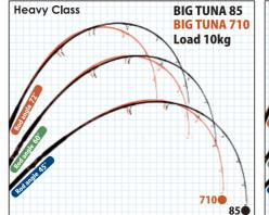
Static load comparison of BIG TUNA 85 & BIG TUNA 710 (10kg load) These two models are the core of the series capable of use with various size lures for different bait sizes. The 85 is an extended model of the 710 with a sharper tip section when casting. Although the long length blank may feel stiffer, the butt section of the 710 is predominantly stronger.
