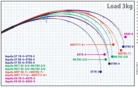
Here are the comparisons of the Aquila series with a static load of 3kg. Aquila series have been categorized ST, MLT, MST and EX.
