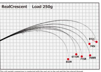
This still weight comparison is conducted with the reel set to the rod and the line placed through each guides to give you a more true comparison. The rods are also secured at the grip end and a section a little higher from the reel foot. These bend curves do not represent all of the rods true characteristics so please take these comparisons just to give you an idea of our lineup.
